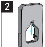
Activate **all** of the refill sensors to remove all the pressurized water in the water station(s).
